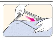
2 Remove vinyl packing of new filter, put into Ag allergy shield filter case so that black
